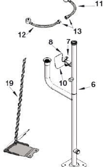
Inlet and Outlet Connections: 25mm BSPM
