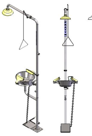
Inlet and Outlet Connections: 25mm BSPM Recommended: Minimum Supply Connection: 25mm Minimum Water Supply: 140-150 LPM @ 210kPa
